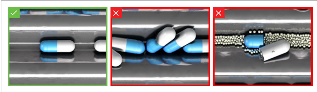
출처 : Cognex, 'How AI and Machine Vision Improve Pharmaceutical Product Quality and Yield'
